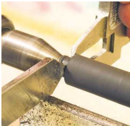
▲ Pic.23 Size the spigot with a parting tool. Les is using a small drive in the headstock so he can get then get the spigot right down to the required 10mm for the hole in the base
